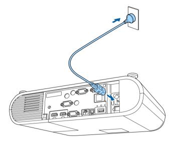
The projector's power indicator turns blue. This indicates that the projector is receiving power, but is not yet turned on (it is in standby mode).
