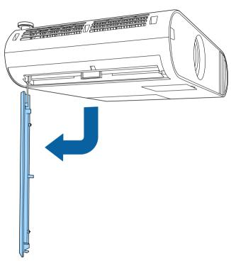
Pull the air filter out of the projector.
