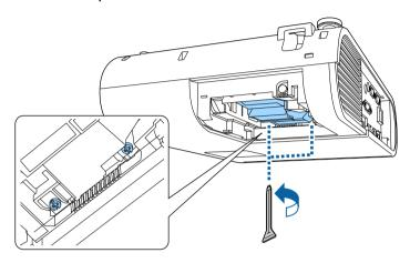
Grip the raised section of the lamp and remove it.
