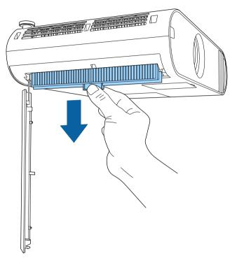
Vacuum both sides of the air filter to remove any remaining dust.
