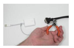
**NOTE:** (On steps #2 and #4) Be sure to use a firm grip with the enclosed crimping tool to fully crimp the metal sleeve.
