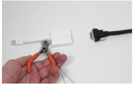
**4)** Slide the metal ring sleeve up tight on the second item, and crimp the metal sleeve securely using the enclosed crimping tool.
