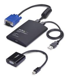
The USB crash cart adapter gives you control of a headless system, turning your laptop into a portable crash cart for rack servers, PCs, ATMs, kiosks, and more.
