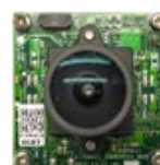
e-CAM50_CUNX - 5.0 MP NVIDIA® Jetson Xavier™ NX/NVIDIA® Jetson Nano™ Camera
